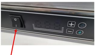
Turn on the roller grill and set the temperature to the lowest setting. This causes the rollers to turn and makes them easier to
