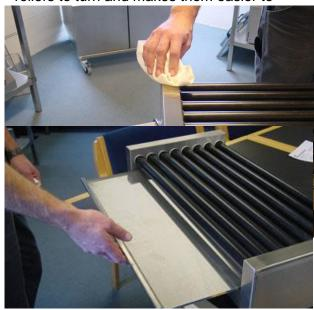
Remove the tray under the rollers and clean it.
