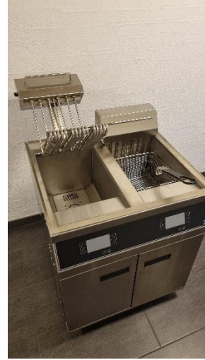
Leave the heating section hanging on the tap during cleaning for easier access to cleaning the vat. Remove the grate and clean it.
