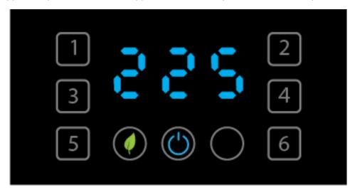
Figure 2, active mode showing the temperature setpoint for the bottom pan at 225°C.
