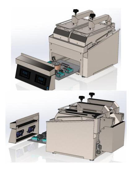
After completing service work on CLAMSHELL GRILL, check and reattach all cables, making sure that they are are secured and will not be trapped by the moving parts. Similarly, the wires attached to the electrical component plate are secured when the plate is gently pushed back into place and the front cabinet is reinstalled.
