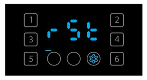
Figure 13, restoring factory settings.
