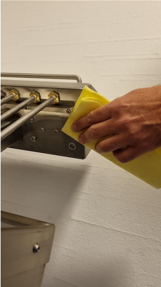
Exercise particular caution in the area near the magnetic contact. Regular cleaning is particularly important here.
