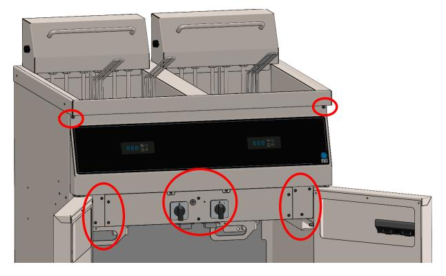
After completing service work on the Fryer STD, check and reattach all cables, making sure that they are are secured and will not be trapped.
