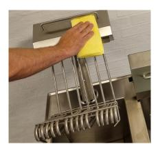
Wipe down the heating section with a damp cloth.
