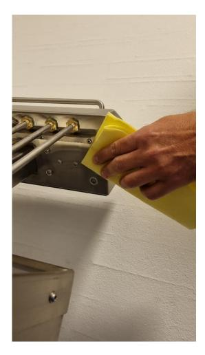
Pay special attention to the area around the magnetic contact, both on the heating section and on the table top. It is important to clean thoroughly here.
