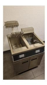
Leave the heating section hanging on the tap during cleaning for easier access to cleaning the vat. Remove the grate and clean it.
