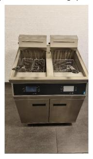
Place the heating section and basket back in position.
