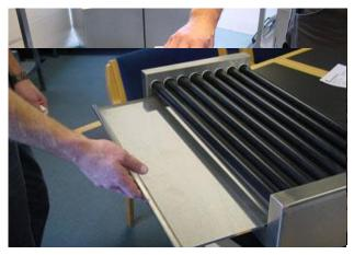
Remove the tray under the rollers and clean it.
