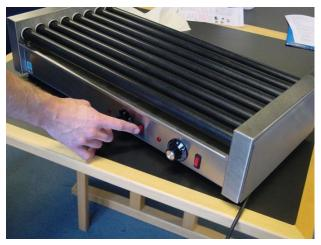
Turn on the Roller Grill and set the temperature to 1. This causes the rollers to turn and makes them easier to clean.
