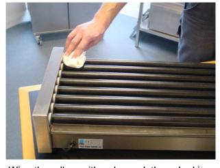
Wipe the rollers with a damp cloth soaked in detergent. Dry inwards towards the centre of the rollers to prevent fat from being pushed back into the cabinet.
