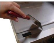
After each frying, the pans must be scraped free of excess fat so that it does not burn, resulting in odor and smoke nuisance. First, scrape excess fat off the upper forehead and then scrape excess fat off the forehead and to the fat drain in front on the left side.
